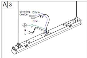
A 3 3. Connect AC wire and dimming wire.
