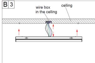
B 3 3. Lift up the fixture and put wires into box.
