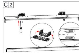
C 2 2. Bend mounting plate, fixed to bottom of the fixture by screws, and then fix it to the installation position.
