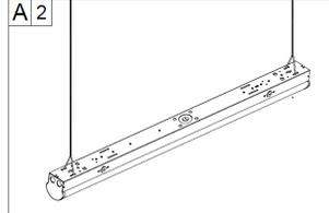
A 2 2. Fix chain to installation location, adjust the height of chain until fixture is balanced.
