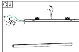
C 3 3. Connect wire. If connect wire at side, please insulate both ends of AC wire at the bottom.
