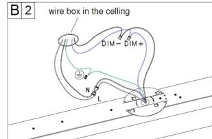
B 2 2. Connect AC wire and dimming wire.
