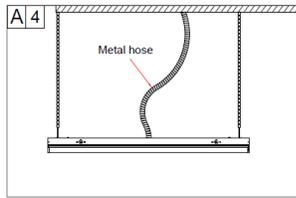
A 4 4. Wrap wires with metal material.
