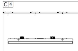
C 4 4. Put the wire back in the box. Multiple fixtures can be installed on a line. But can not be connected to more than 10 fixtures because of limited wire load.
