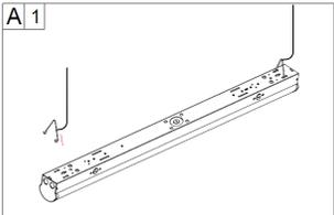
A 1 1. Tie hook with chain (or wirerope) and then insert it into installation hole.
