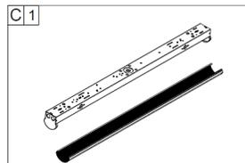
C 1 1. Lateral movement and remove the diffuser.
