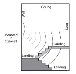
Features Time Delay: 5 to 30 minutes Coverage at 8' height, 24' diameter
