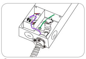
6 Connect the AC mains power to LED Driver, for 0-10V dimmable panel, connnect the 0-10V dimming cable.
