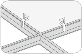
4 Check the clips well fasten to T-BAR(Main/Cross ceiling tee).
