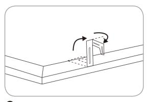
2 Lift the mounting clip on the edge of panel. Turn the mounting clip head
