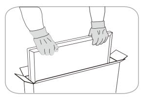
1 Take the panel out of the box and protective bag, Remove the protective film.
