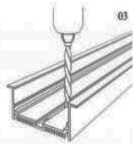
03 Drill hole for power cord.
